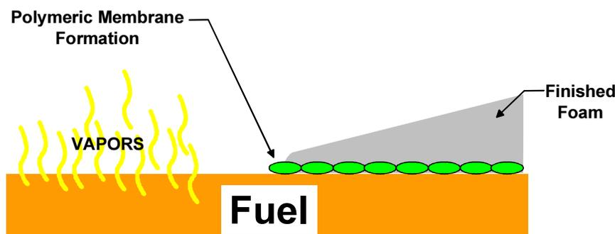
AFFF's are a combination of fluorochemical surfactants and synthetic foaming agents. AFFF's extinguish fires by forming an aqueous film. This film is a thin layer of foam solution that spreads rapidly across the surface of a hydrocarbon fuel causing dramatic fire knockdown. The aqueous film is produced by the action of the fluorochemical surfactant reducing the surface tension of the foam solution to a point where the solution can actually be supported on the surface of the hydrocarbon.
